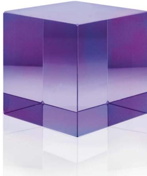
Calcium fluoride single crystals, grown from high purity raw materials, are required for illumination and projection optics in 248 and 193 nm micro-lithography technologies.
