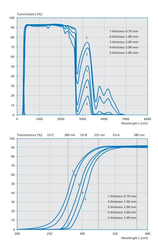
BOROFLOAT<sup>®</sup> 33 – Transmittance in the UV Range
