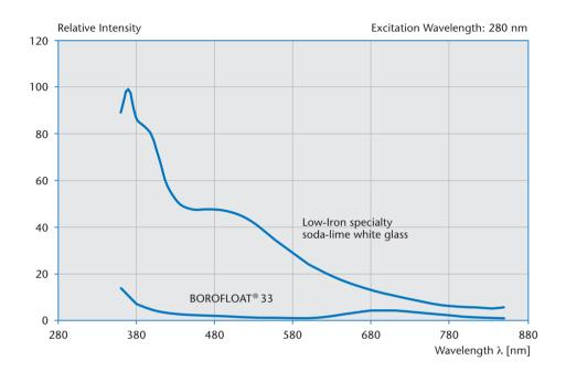
Fluorescence Behavior of BOROFLOAT<sup>®</sup> 33 and Soda-Lime Glass Type for Different Wavelength Excitation
