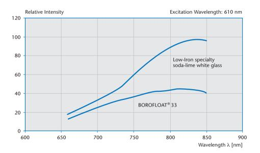
Fluorescence Behavior of BOROFLOAT® 33 and Soda-Lime Glass Type for Different Wavelength Excitation
