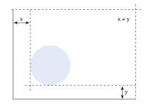
Permitted borehole position deviation: Deviation of borehole center: ± 1.5 mm.
